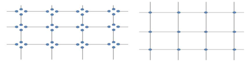
An HVDC Grid is defined in Cigre as an HVDC system consisting of at least three converter stations and at least one mesh formed by transmission lines.
